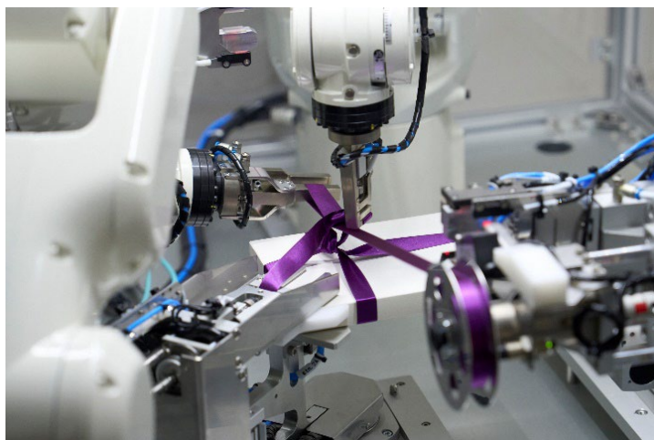
Examples of equipment developed by Abilica: Automatic ribbon-tie tying machine for gift boxes
