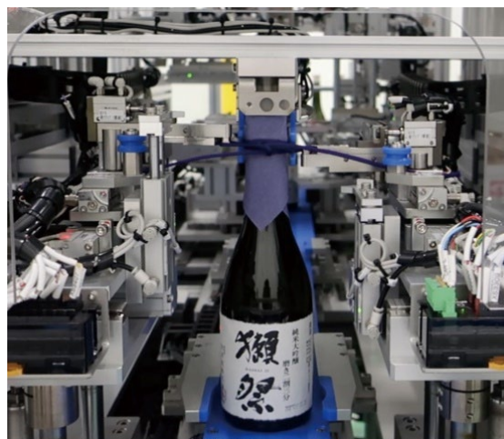
Automatic bottle decoration machine for sake bottles
